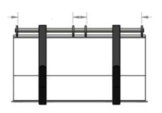
**MOUNTING BRACKETS** 3/8" THICK require 1/4" **FILLET WELDS** down both sides.
